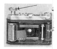
the camera. Turn the knurled reel flange to bind the film on the reel until the full width of the film just emerges from the magazine. After making sure that the film will ride properly in the path provided for it, close and lock the back of the camera and turn the winding knob in the direction of the arrow until it locks.
