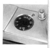
**4.** Turn the exposure counter, by means of the two small studs, until the figure 20 (for a 20-exposure roll) or the figure 36 (for a 36-exposure roll) is at the index mark. The counter will always show the number of exposures remaining on the film.
